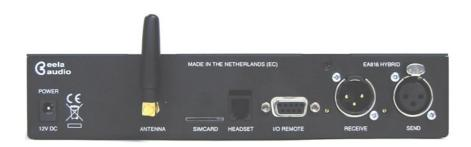
LINE INPUT: On XLR type connector the balanced line input of the unit.
